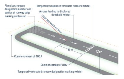
Markings for a temporarily displaced threshold due to works on the runway for a period in excess of 30 days
