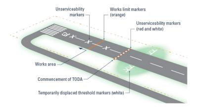
Markings for a temporarily displaced threshold due to obstacle infringement of the approach path for a period in excess of 30 days
