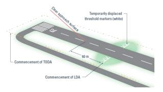
Markings for a temporarily displaced threshold due to works on the runway for a period of 30 days or less
